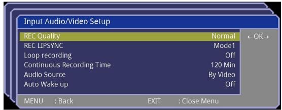
♠ REC Quality: Sets the video compression bit rate, which can be Excellent, High, Fine, Normal or Basic. Approximately 4 GB storage are needed to record 60 minutes of HD video, using the Normal setting (see table below):
