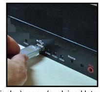
utility in the HDTV Recorder's OSD (On Screen Display) menu (explained later). **Note**: You must always plug in the USB storage device before turning on the HDTV Recorder. Also, you should power down the HDTV Recorder before detaching the USB device.
