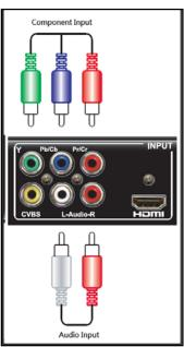
c) **CVBS**– The CVBS cable is a single cable with a video connector (usually yellow). You will also need to attach two audio connectors (for L-R speakers, usually red and white). The CVBS cable may come as a single cable with the 3 connectors at each end. Attach the other ends to your Video Player.
