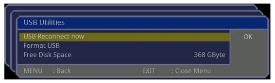
The "Format USB" item can be used to format a USB HDD, a USB Pen drive or a memory card used with a USB card reader. The HDTV Recorder formats using the FAT/FAT32 file system format. (HDTV Recorder does NOT support other file systems).
