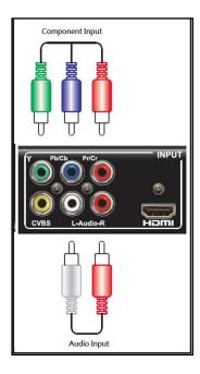
c) CVBS— The CVBS cable is a single cable with a video connector (usually yellow). You will also need to attach two audio connectors (for L-R speakers, usually red and white). The CVBS cable may come as a single cable with the 3 connectors at each end. Attach the other ends to your Video Player.
