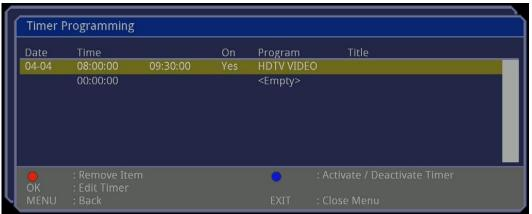
After you save your new recording schedule session, it will appear in the Timer Programming list. The system will automatically awaken and begin recording when the "Start Time" arrives. You can press the button to delete an item, press the button to enable or disable an item, or press the button to edit an item. The button will return you to the previous OSD
