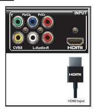
b) YPbPr – YPbPr cables have 3 connectors, each color coded (green, blue and red). Simply match the colors on the connectors with the color coded adapters on the AnyHD Recorder (top row - shown right).
