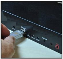
**Note**: You must always plug in the USB storage device before turning on the AnyHD Recorder. Also, you should power down the AnyHD Recorder before detaching the USB device.
