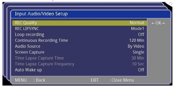
♠ REC Quality: Sets the video compression bit rate, which can be HIGH, FINE, NORMAL or BASIC. Choosing HIGH will use the maximum video bit rate. The BASIC mode will use the minimum video bit rate. Approximately 4 GB storage are needed to record 60 minutes of HD video, using the NORMAL setting (see table below):
